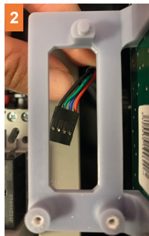
2 Locate the VSP cable and position it as shown in the photo (red on the right) ■■■■■■
