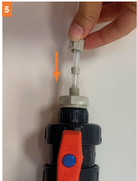
5 Push the rigid tubing into the valve adapter.
