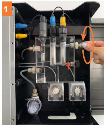
1 Unscrew the connector from the outlet union
