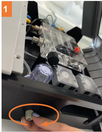
1 Unscrew the connector from inlet union (pre-filter connection)
