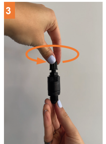
3 Unscrew the connector from the injector.
