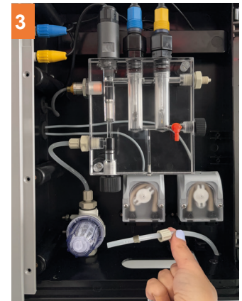
3 Fit the connector and ferrule onto the rigid (white) tubing. Make sure the orientation of the two parts is as shown in the photo. Part B (ferrule) is inside part A (connector).
