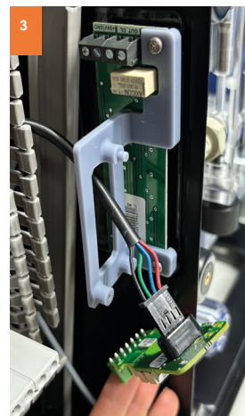
3 Connect the VSP driver pins to the VSP cable. Make sure the connector and pins are positioned correctly ■■■■■■
