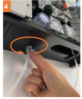
4 Screw on the connector and check that the tubing has been tightened correctly
