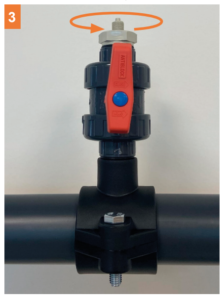
3 Approx. 8 turns of Teflon should be applied to the thread of part C before screwing it into valve D.
