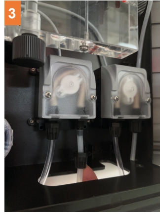
3 Push the rigid tubing into the pump's outlet union
