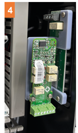
4 Tighten the two screws and press at the top of the driver to secure it and close the cable channel
