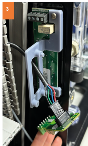
3 Connect the VSP driver pins to the VSP cable. Make sure the connector and pins are positioned correctly ■■■■■■
